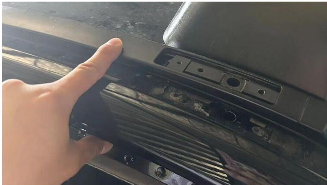
2. Put the Roof rack on the roof strip, corresponding position cut off the unwanted parts of the strip.
