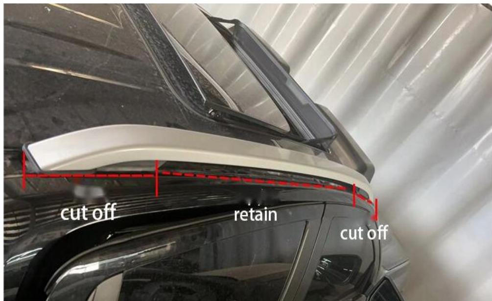
3. Install the retained strip back into place.
