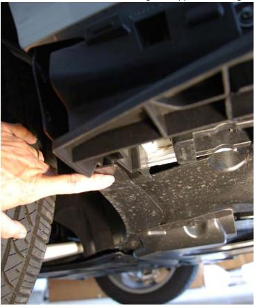
8. Install running board. Caution: Be sure that the running board goes BEHIND the existing mud shield.
